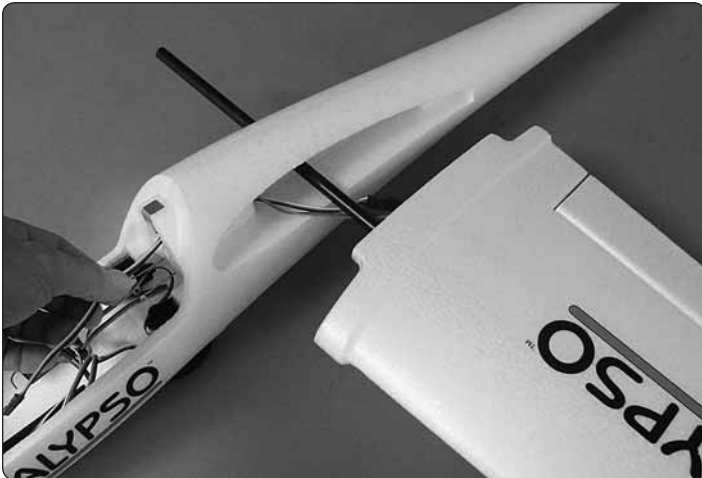
❑ 4. Insert the wing into the fuselage as you guide the servo wires through.
